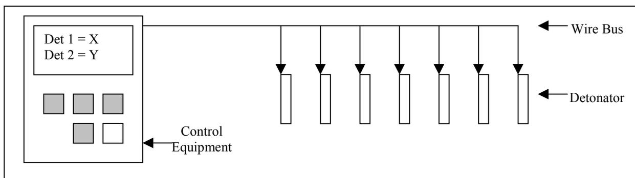
**Figure 1. A Basic Electronic Detonator Control System**
