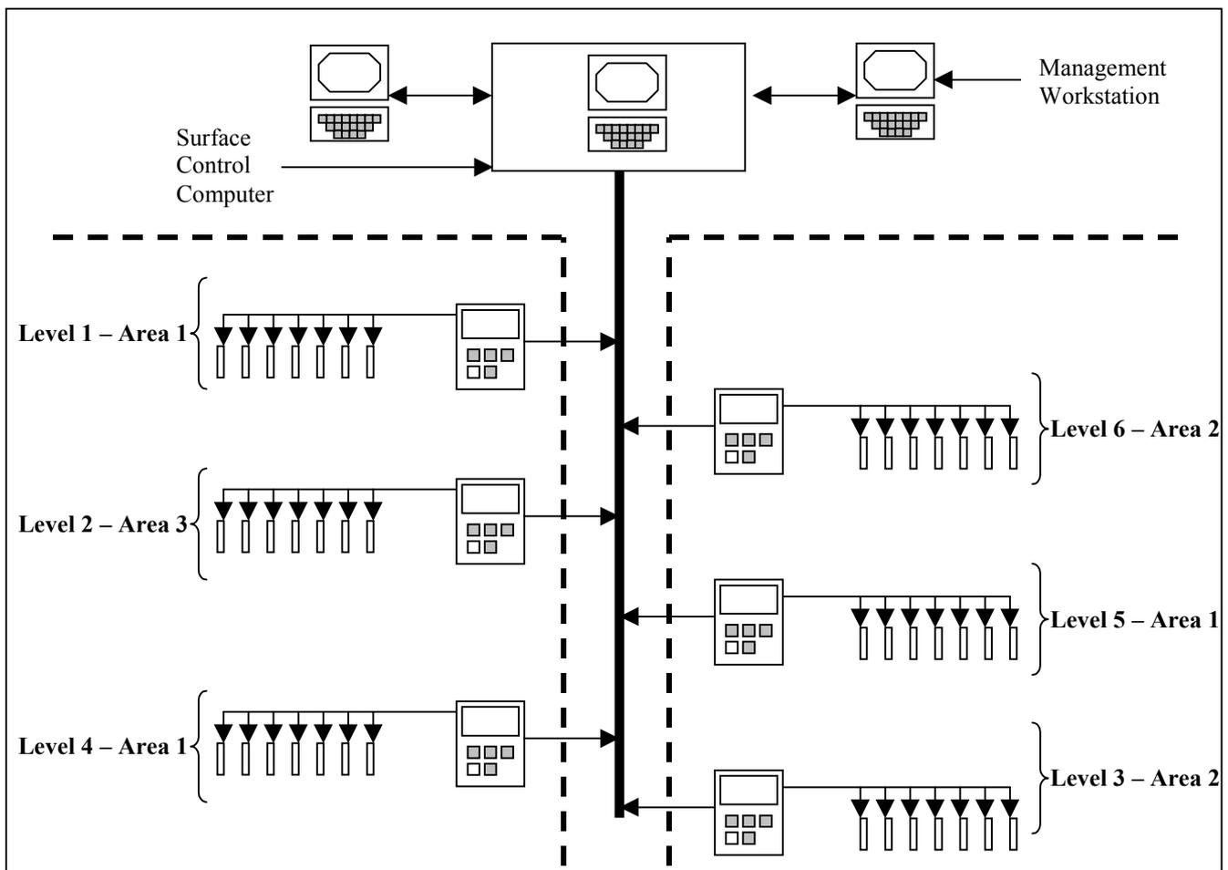
Figure 2. The Modern Blast Control Network
